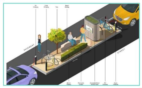
Figure 13 – Visualisation of a small-scale Plymouth mobility hub<sup>17</sup>
